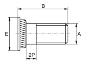
For plate thickness, min = 1.5 Head diameter E = 6 Hole diameter +0.1 = 4.2 Length B = 10 Male thread A = M3x0,5 Min distance to edge = 2.4
